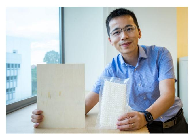
Made out of interlocking eight faced octahedrons that are wrapped in plastic, the structure becomes 25 times stiffer when vacuum packed. Similar to how your loose grains of coffee become a rigid mass when vacuum packed, the stiffer packed structure can actually act as a form of armor.
